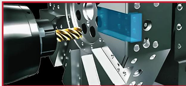
On-The-Fly Indexing - This standard feature allows tool changes on the fly as the axes retract from the part. Combined with high-speed rapid movements, this results in faster tool changes and shorter cycle times by reducing non-cutting time.
