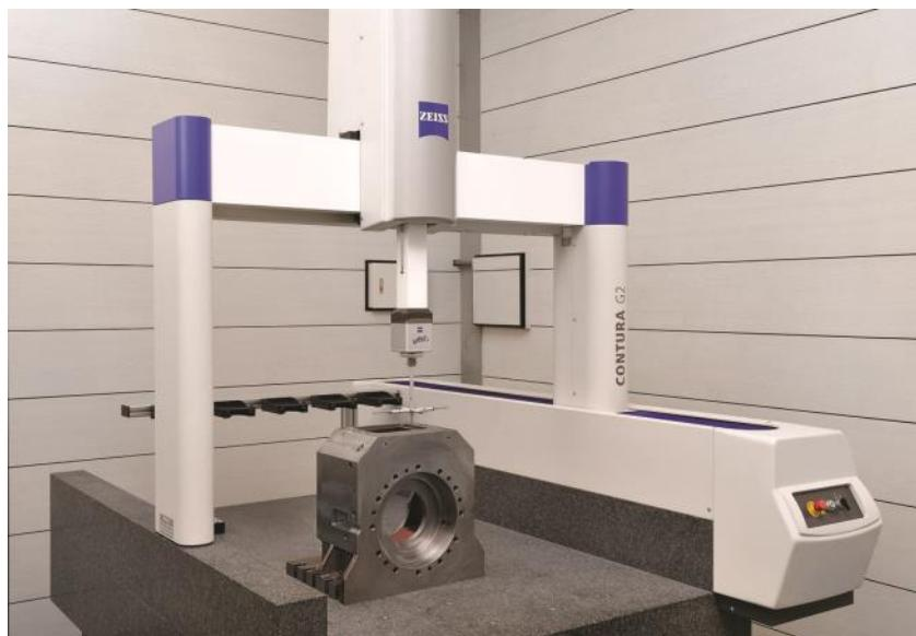
ZEISS CMM for components inspection
